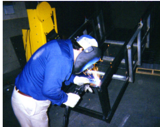
Figure: An Ergo Control optimizes the position of the product for the worker.
